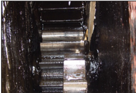
Exposed gear teeth and hard residues.
